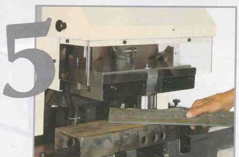
PRESS STATIONS 20 TONS forming • straightening • mounting various (tooling option)
